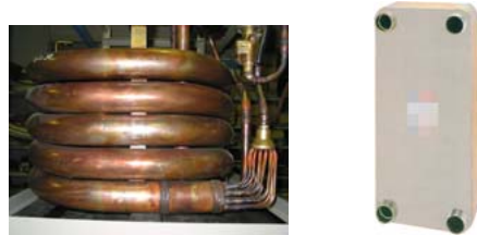
Fig. 1. Heat exchangers (Left: Conventional copper multiplex pipes, Right: SUS plates adopted newly)
