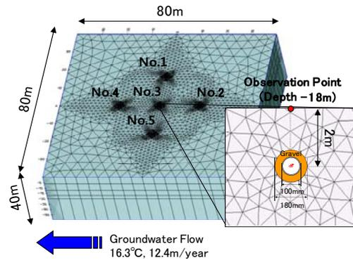
Fig. 7. Simulation model
