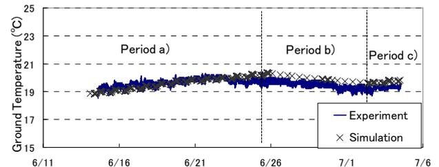
Fig. 8. Comparison of simulation and experiment result results. During period a), the groundwater temperature slightly increases by discharging heat at return well but during period b), in which ambient air is used as a heat source, it decreases gradually. The simulation result shows fairly good agreement with the experiment result.
