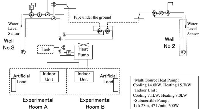
Fig. 3. System configuration
