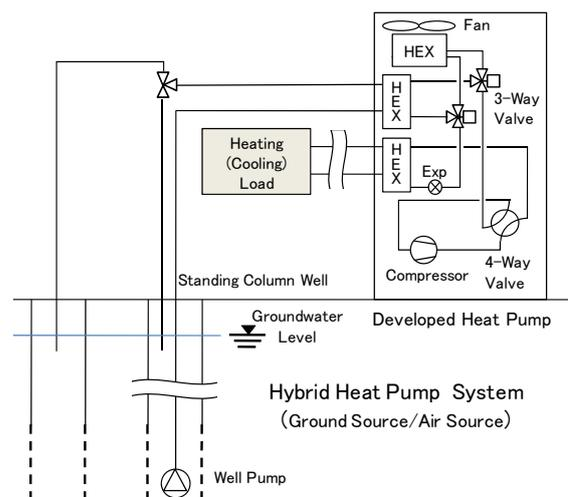
Fig. 1. Image of developed system
