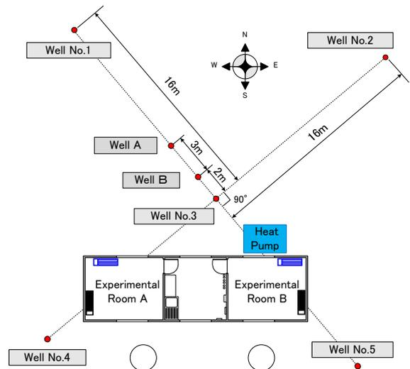
Fig. 2. Layout plan of experimental equipments
